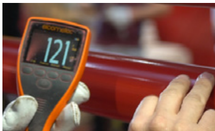
Adherence and layer thickness test.
