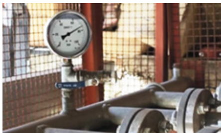
Hydrostatic pressure test. 5 min 80 bar.
