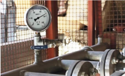
Hydrostatic pressure test. 5 min 80 bares
