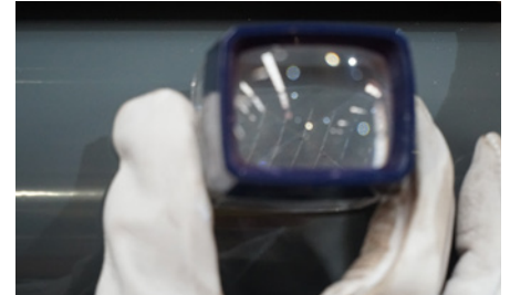
Polyester powder coating adherence test
