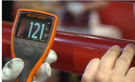
Adherence and layer thickness test
